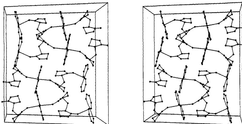
**Figure 2.** Stereoscopic view of the unit cell contents, projected down the  $c$  axis. The  $+a$  direction is to the left, and  $+b$  points downward. For clarity,  $\text{CF}_3$  and  $\text{CH}_3$  groups have been omitted.
